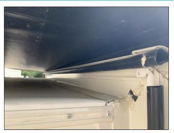
Slideout Roof Bulb Seal
