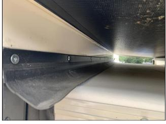
Slideout Roof Sweep Seal
